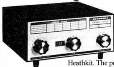
HX 1681 CW Transmitter. Full break-in CW operation. Built-in VFO. Covers 80 through 10 metres CW. Rugged 6J46A finals give 100W on 80-15M, 75W on 10M.
